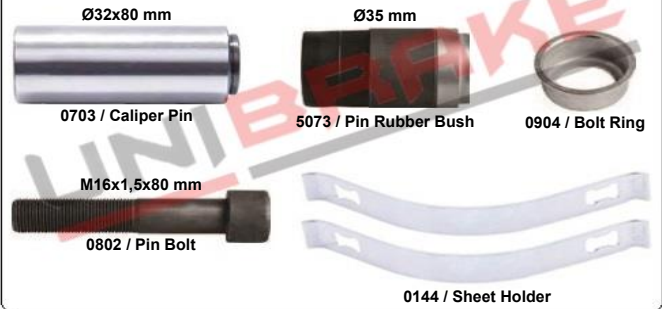
5194 / Caliper Repair Kit SB6 / SB7 Type KNORR: K000421
