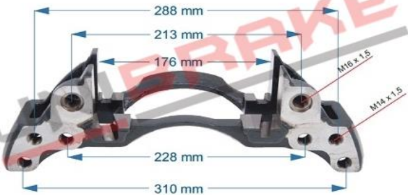
6803 / Caliper Carrier / 12-153 MAN - LEFT WABCO CARRIER
