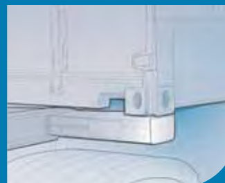
RECOLOCK® locks the container firmly on the trailer
