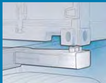
The corner casting and locking mechanism fit together perfectly
