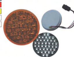
TD04-68-010 UNIVERSAL TAIL LAMP WITH 40 LED SIZE:ø4"×1.1"
