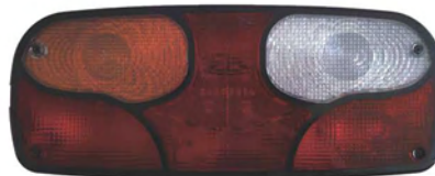
TD02-63-004 UNIVERSAL TAIL LAMP LH WITH NUMBER PLATE: A252000507 RH NO NUMBER PLATE: A252400507 LENS: A188520002
