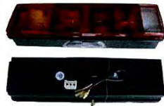
TD-52-005 SCANIA R142 P113 TAIL LAMP OEM NO.A:LH WITH LICENSE LAMP 1365963 A:RH WITH LICENSE LAMP 1365966 B:LH NO LICENSE LAMP 1365965 B:RH NO LICENSE LAMP 1365964
