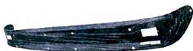
TD-51-088 VOLVO FM12 FH12 SUN VISOR PRESSING OEM NO.1619092(TWO HOLES) 8140923(NO HOLES)
