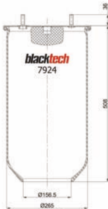
RML 7924 Air spring system without piston
