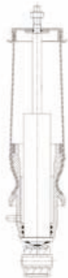
110 01 CA Cabin air spring with shock absorber plates
