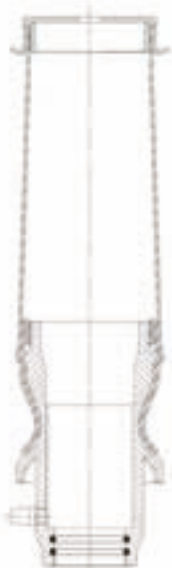
110 01 C Cabin air spring without shock absorber
